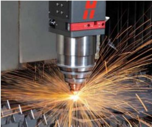
3 kW fiber-based cutting laser (Hypertherm)
